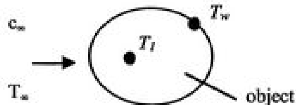
Temperature variation in an object cooled by a flowing liquid
