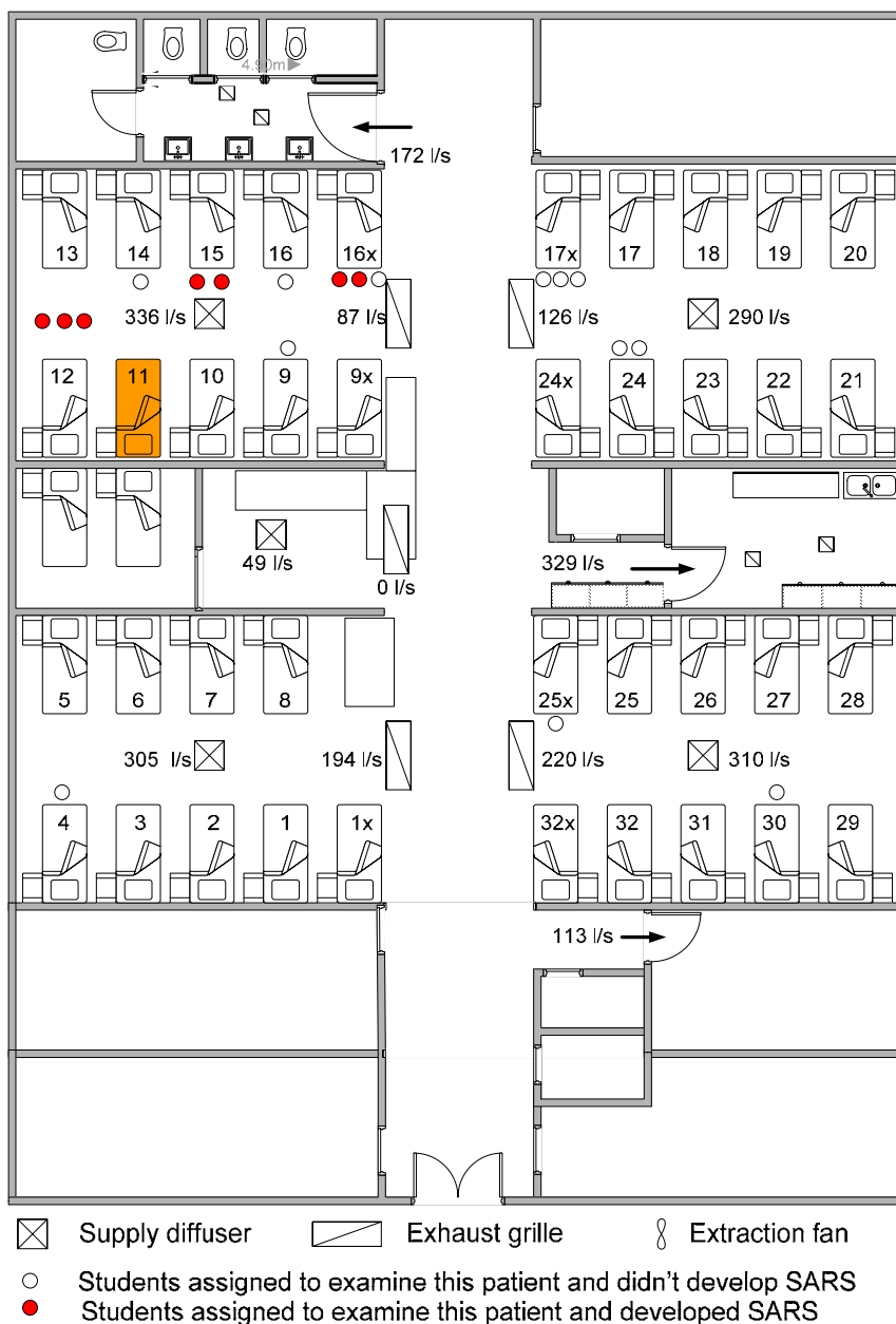
Figure 1 Floor plan of Ward 8A at the time of outbreak in March 2003. Measured supply and exhaust flow rates are also given. The bed no.11 where the index patient stayed is highlighted. The locations of the 19 medical students who attended the 40-min bedside clinical assessments are also highlighted. (Modified from [5]).
