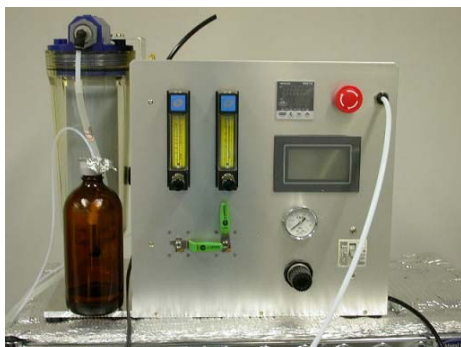
Photo.1 The pollutant constant-emission device of instantaneous evaporation type
